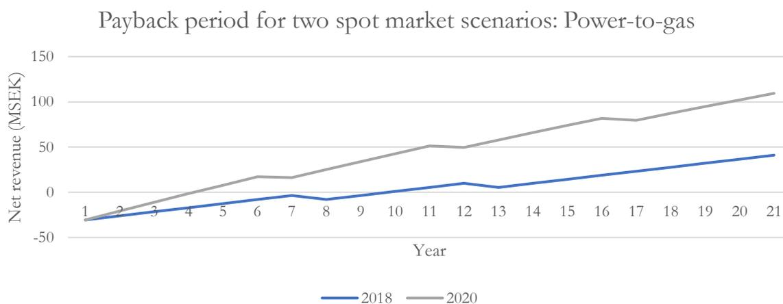
Figure 13 - Payback period of the power-to-gas system
