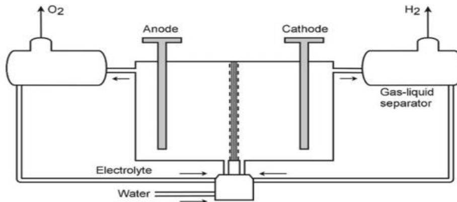
Figure 3 - Schematic of an AEL cell (Bailera, M., Lisbona Martín, M.P., Peña, B., Romeo, 2020)
