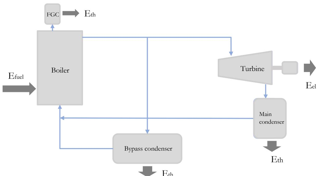
Figure 2 - Schematic of Igelsta Combined heat and power plant. The blue lines represent the water/steam flow and the gray pointers show the energy in and output.
