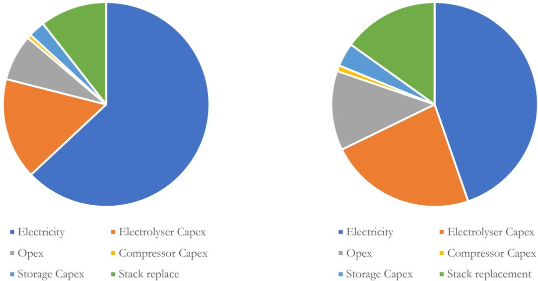
Figure 14 - Life cycle cost of the power-to-gas system for two different years at an electrolyser CAPEX of 10 MSEK/MW.
