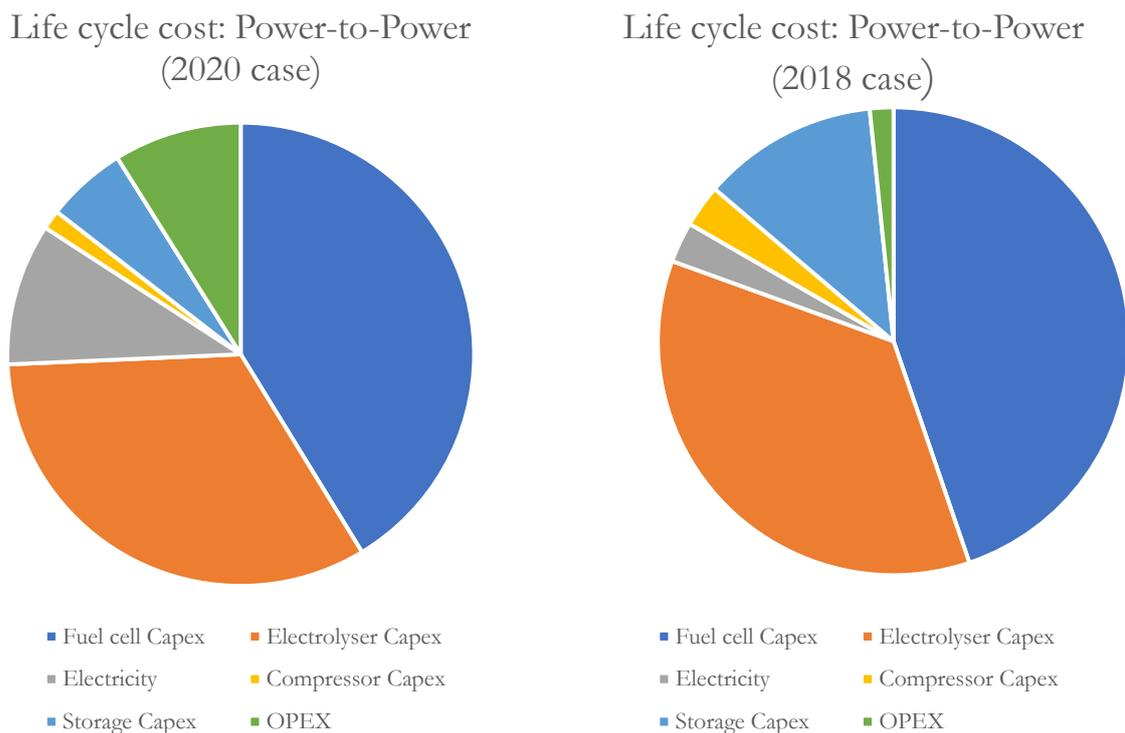
Figure 17 – Breakdown of life cycle costs of the PtP-system at for two examined years. Values are based on fuel cell CAPEX of 15 MSEK/MW and electrolyser CAPEX of 10 MSEK/MW.
