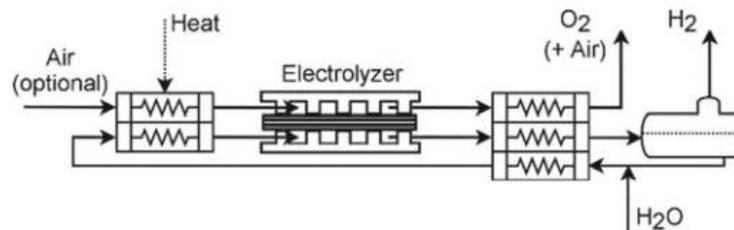
Figure 5 - Schematic of a SOEL cell (Bailera, M., Lisbona Martín, M.P., Peña, B., Romeo, 2020)
