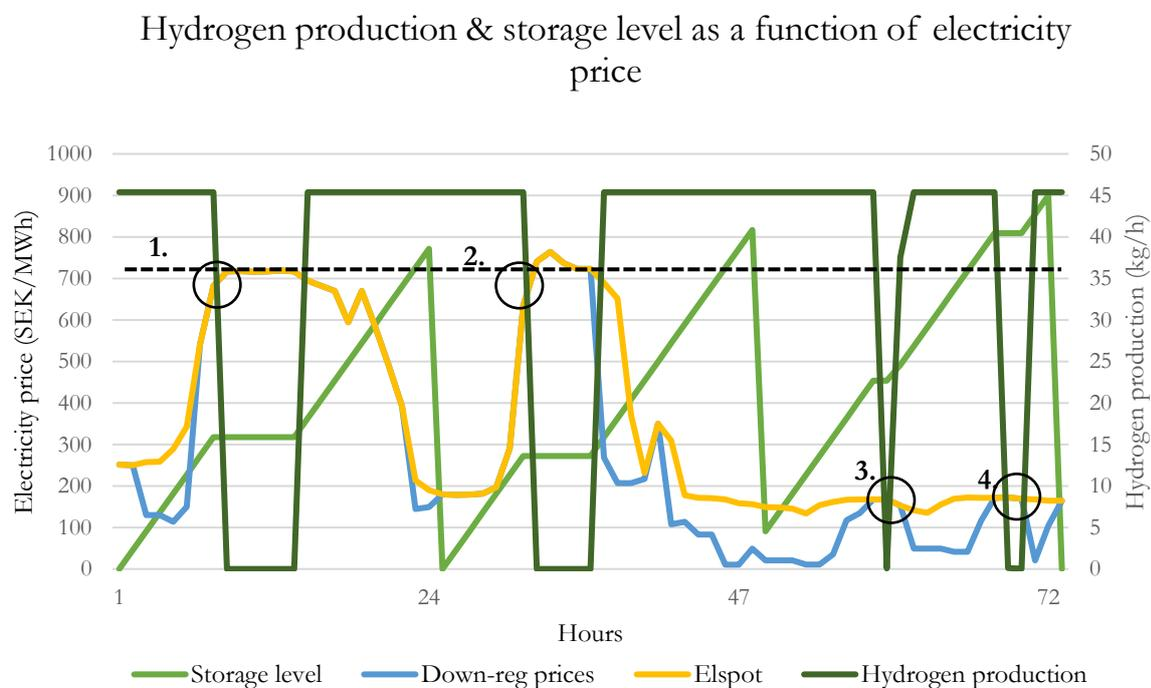
Figure 12 – Example of three days of power-to-gas operation as a function of electricity prices and storage capacity. At 1 and 2, the down-regulating price reaches the breakpoint of 720 SEK/MWh, and the electrolyser shuts down for the high-priced hours. At 3 and 4 the electrolyser pauses its production at the peak-priced hours to cost-optimally fill up the storage.
