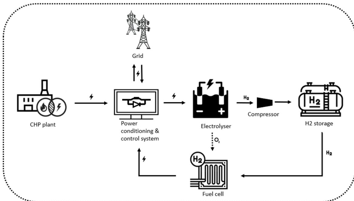
Figure 11 - Schematic of a Power-to-Power system
