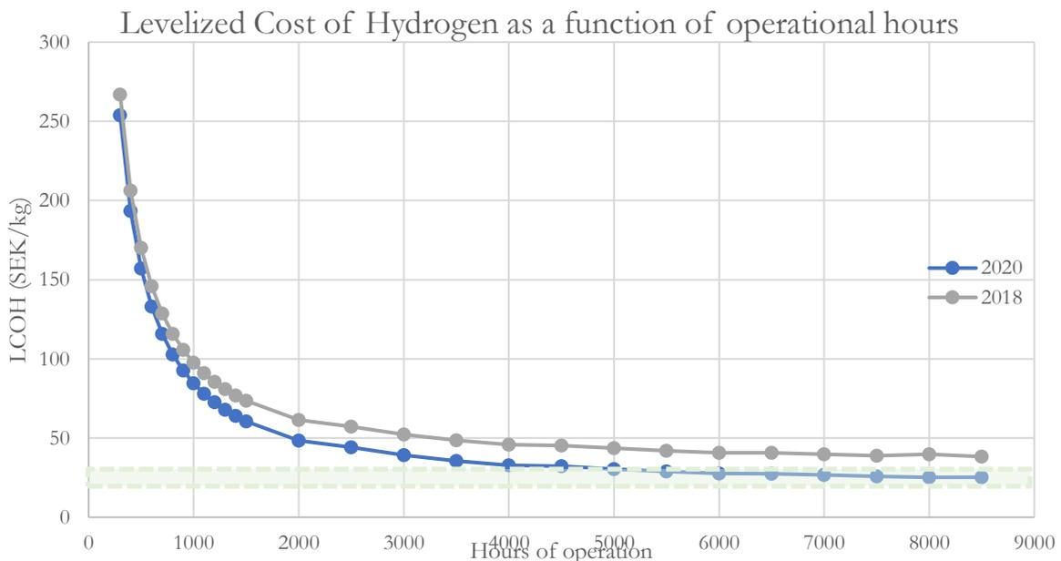
Figure 15 - LCOH as a function of operational hours. Values are based on a electrolyser CAPEX of 10 MSEK/MW. The green area represents the cost range of SMR-produced hydrogen, which is estimated at 15-30 SEK/kg.
