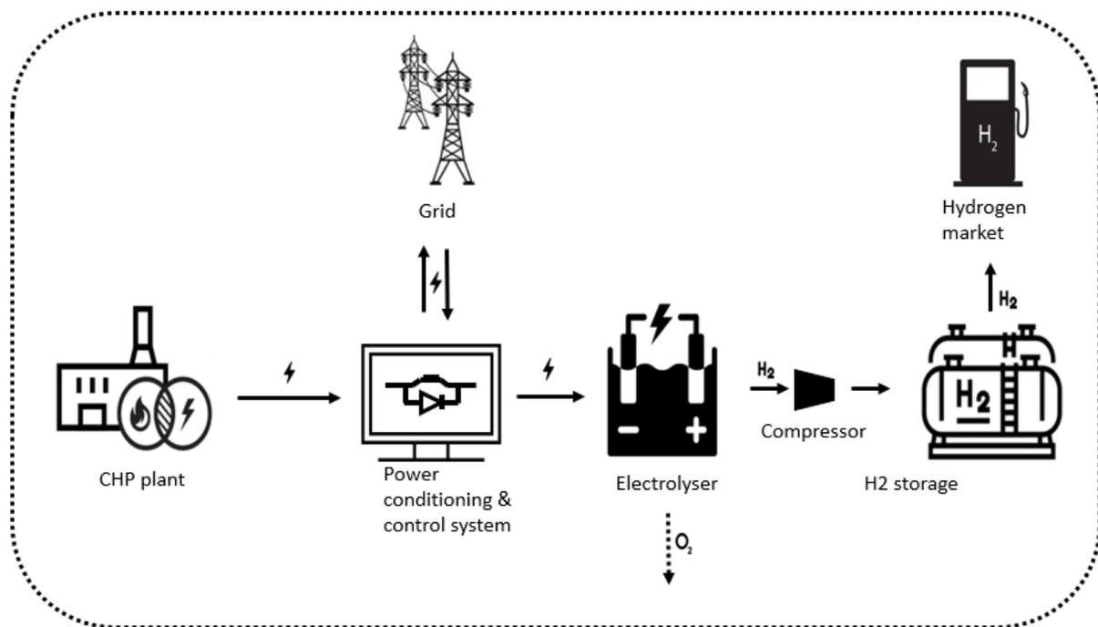
Figure 10 - Schematic of a Power-to-gas system
