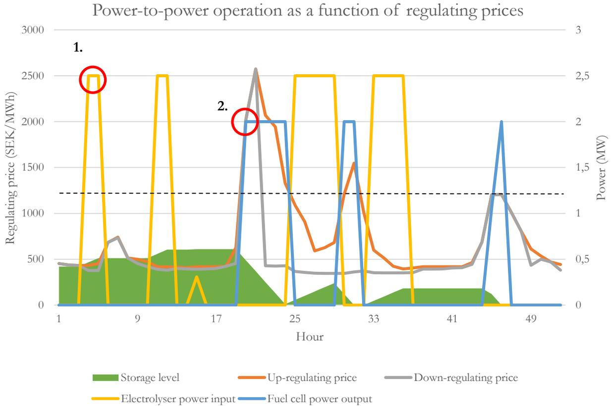
Figure 16 - Example of how the power-to-power system is operating as a function of regulating prices. In point 1, along the yellow line shows the operation of the electrolyser, which activates when down-regulating prices drop. Point 2 along with the blue line depicts the fuel cell activity, which is operational at up-regulating prices over 1200 SEK/MWh.
