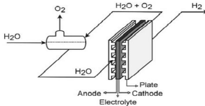
Figure 4 - Schematic of a PEM cell (Bailera, M., Lisbona Martín, M.P., Peña, B., Romeo, 2020)
